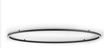
Ceiling or wall lighting fixture for interiors, with direct light emission. Bended extruded aluminium structure in white, black or mat brass polyacrylic paint. Extruded polycarbonate diffuser with opaline finish. Turned brass ceiling-fastening spacers in polyacrylic paint.
